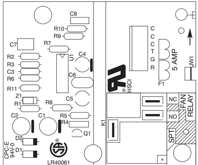
**Fig. 9 - Fan Coil Printed Circuit Board for FY4A Model**
