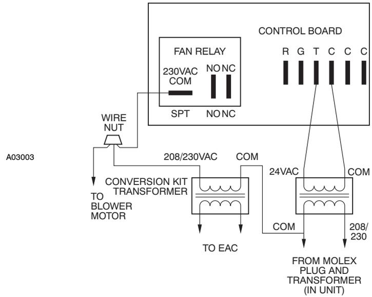
**Fig. 22 - Wiring Layout of Electronic Air Cleaner to Fan Coil for FY4A Models Only**
