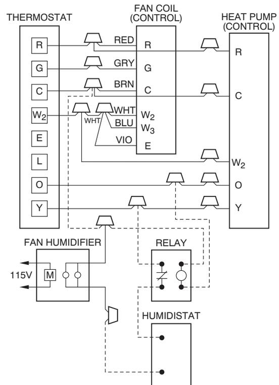
**Fig. 23 - Wiring Layout of Humidifier to Heat Pump**
