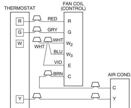
**Fig. 11 - Wiring Layout Air Conditioning Unit (Cooling Only)**
