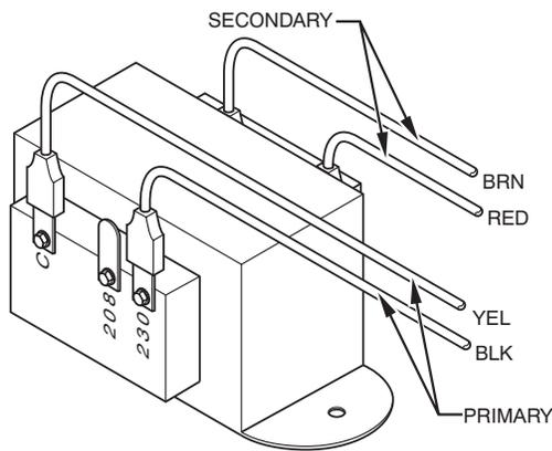
Fig. 17 - Transformer Connections
